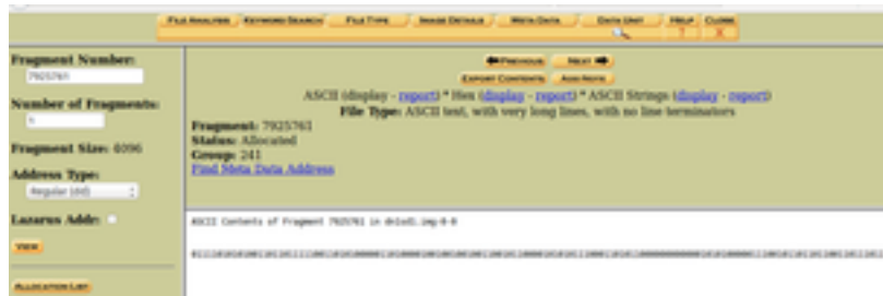
Figure 12: Autopsy recovers the deleted blocks from one of the DataNodes.
